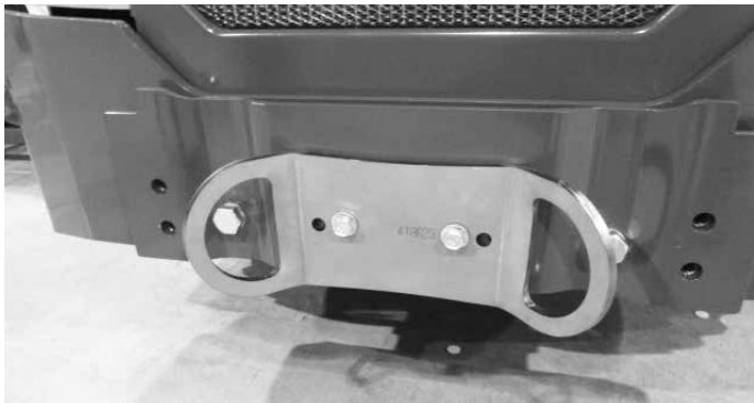
Tie down bracket A418623 installed at the rear bumper or counterweight
